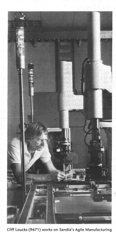
Prototyping System (AMPS), a modular system of manufacturing hardware and software tools enhanced with Sandia-developed sensor and automation software technologies. Together the system comprises a flexible production line capable of assembling a range of electromechanical products. AMPS is available to industry partners for validation of a variety of agile manufacturing approaches.
